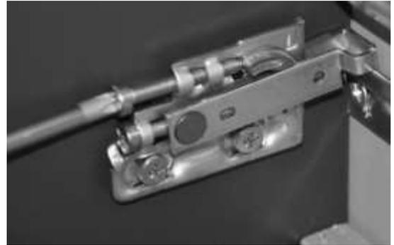
c\_ Now proceed to the leveling of the cabinet by turning the upper screw on the hardware, as shown.
